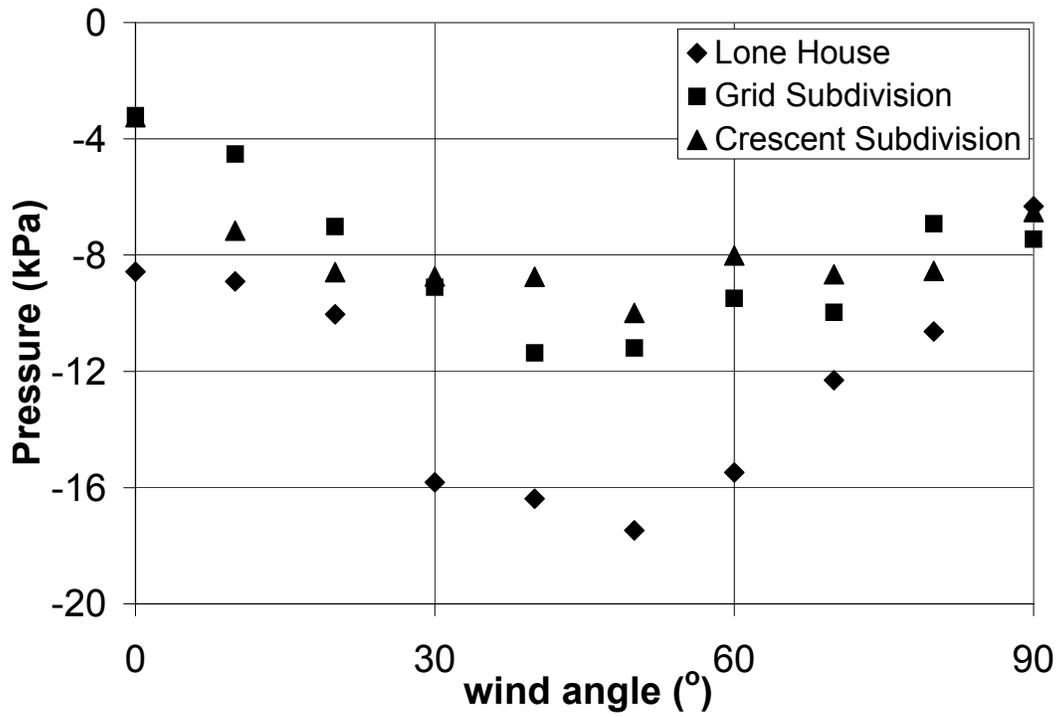
Figure 9. Ridge pressures (kPa) for cladding design in London Ontario
