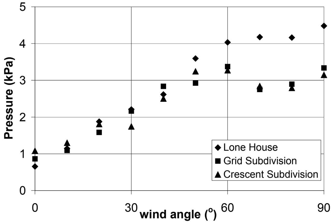
Figure 7. Side wall pressures (kPa) for cladding design in London Ontario.
