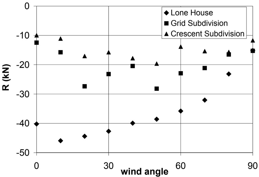
Figure 10. Peak vertical end reaction (kN) at Truss 1 for London, Ontario.
