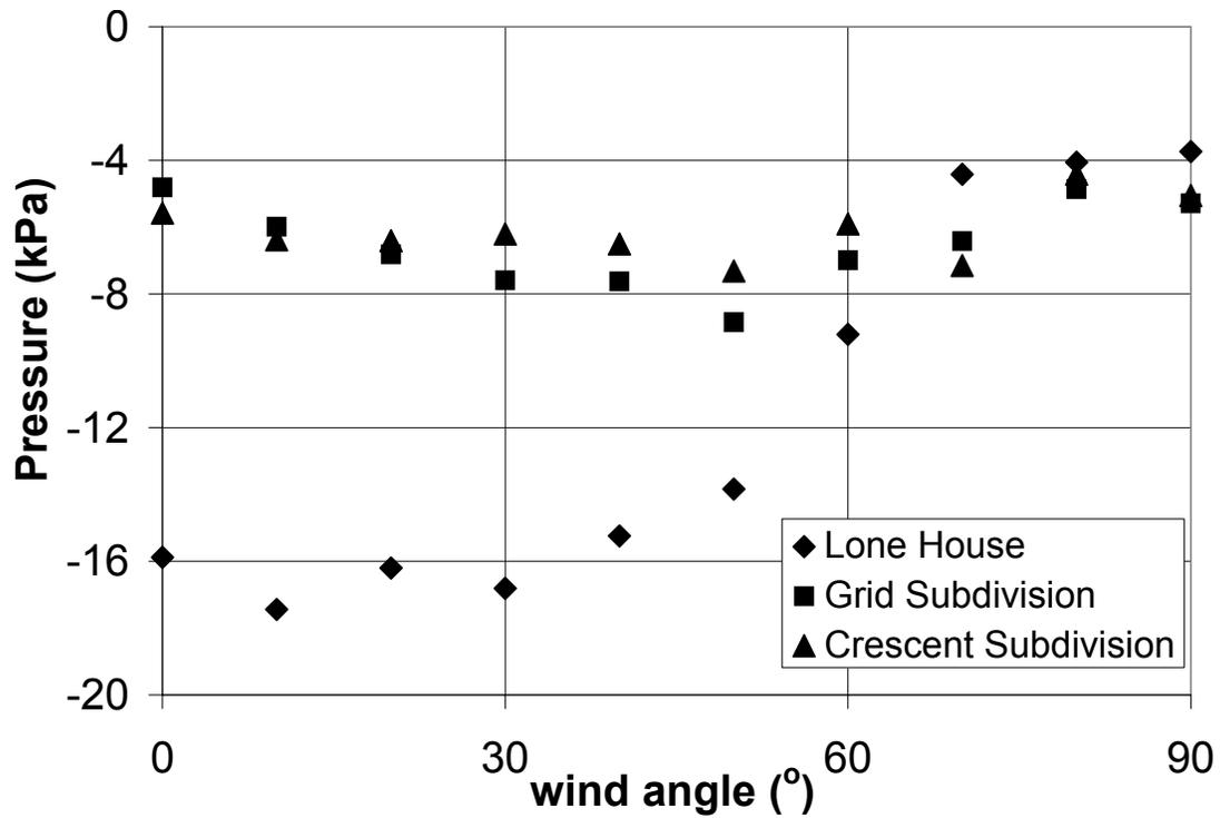
Figure 8. Roof corner pressures (kPa) for cladding design in London Ontario.
