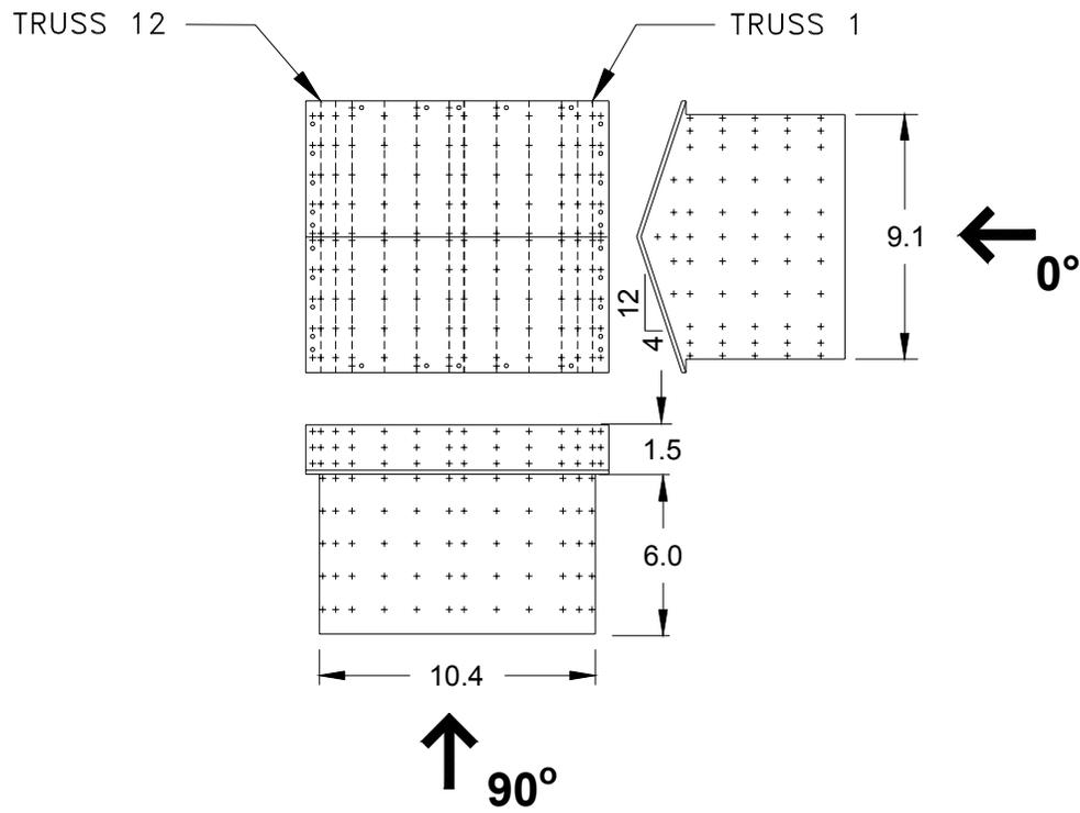
Figure 5. Exploded view of wind tunnel model, illustrating pressure tap and assumed truss locations. All dimensions are in full-scale metres.
