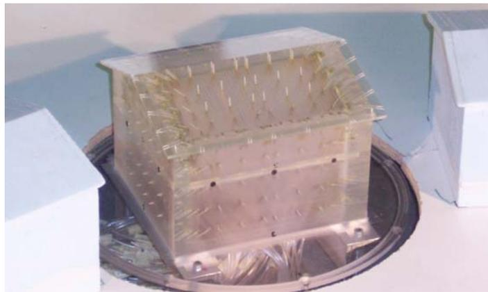
Figure 3. Instrumented wind tunnel model used in the current study.
