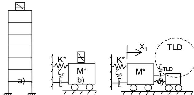
Fig.2 a) Structure-TLD b) Equivalent Representation c) TMD Analogy
