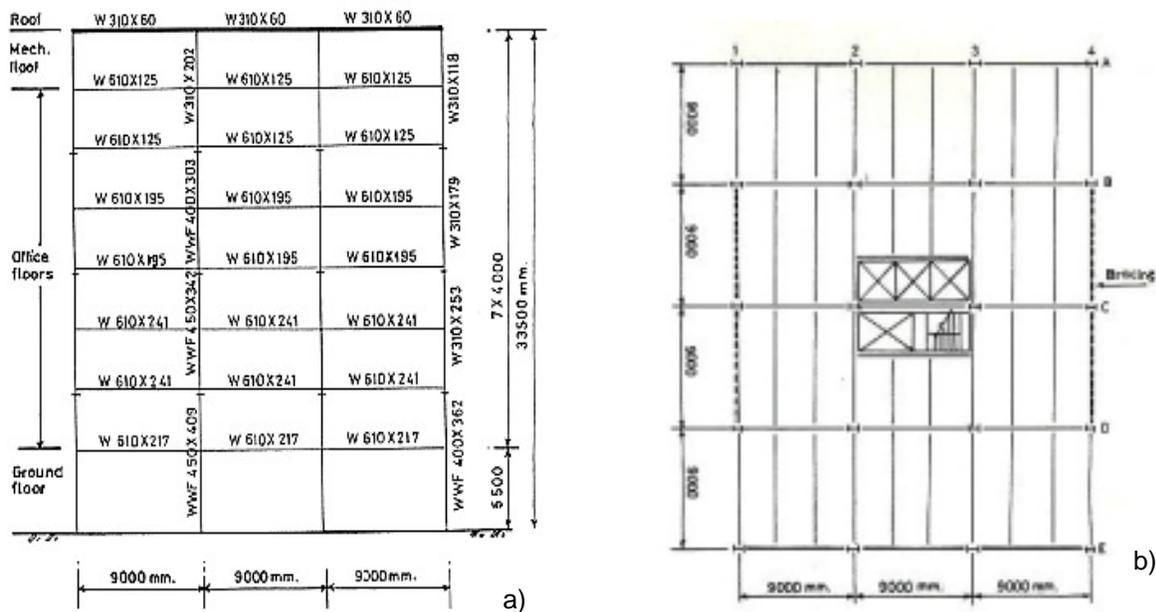
Fig 4 a) Elevation with cross sections and dimensions b) plan
