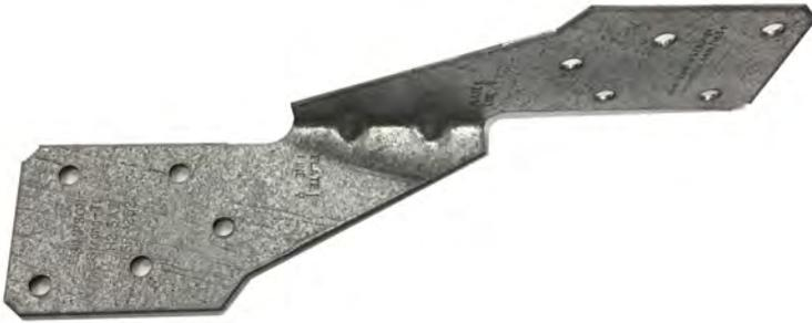
**Figure 19:** Hurricane ties, including clips, are strips of metal that are engineered to bind the roof rafters or trusses to the top plate of a wall. (Source: IPSC)
