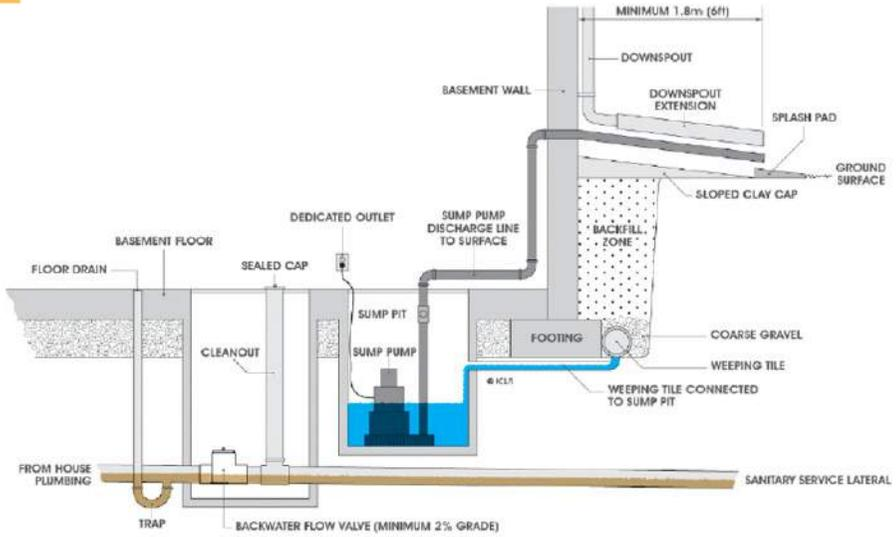
Figure 19 : Installation of a backwater valve
