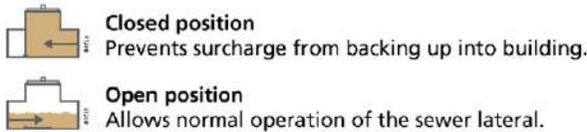
Figure 20 : Backwater valves in open and closed position
